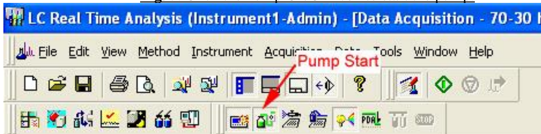
Fig. 5. Click the Pump On/Off icon to start the pump.
